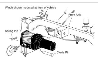
Fig. 2 Winch Mounted to Vehicle
